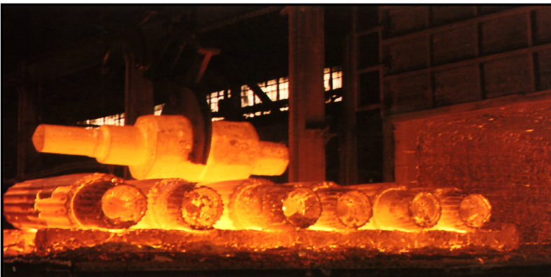
Steel ingots heated to ~ 1600 degrees Fahrenheit
